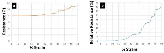
Figure 5. (a) Resistance versus % strain plot (a) and % increase in resistance versus % strain plot for conductive knitted sample. Distance between the two gauges was 3.5 cm. Thus, initial resistance of the sample was 2.3  $\Omega$ /cm.
