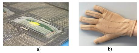
Figure 2. samples of textiles with integrated sensor yarn a) into a flat structure b) into a 3D-structure
