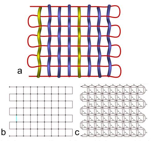
**Figure 4.** Simulated woven structure and its automatically generated cicruits a) 3D geometrical model based on the TexMind Weaver b) circuit for the case of conductive yarns c) circuit for yarns with non negligible resistance
