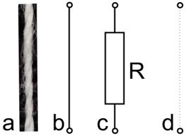
**Figure 1.** Textile yarn and its equivalents in the electric curcuits a) staple fiber yarn b) representation as connecting wire without resistance c) representation as wire with some resistance d) isolator – the yarn does not need to be represented in the system
