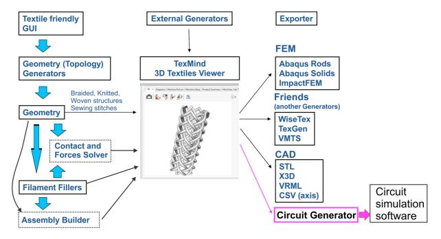
Figure 3. Structure of the software packages for automatic circuit generation.
