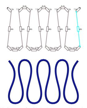
Figure 6. 3D Model of one row of weft knitted structure and its equivalent electric circuit
