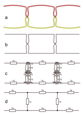
**Figure 7.** Sewing stitch and its circuits. a) 3D geometrical model b) electric equivalent in case of conductive yarns, c) automatically created equivalent circuit based on the contact information d) manually adjusted circuit, based on the automatically created one
