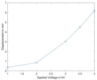
Figure 5. Displacement of the actuated bending beam for actuation voltages between 1 and 4 kV
