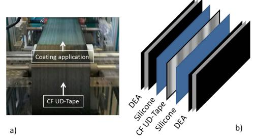
Figure 2. a) Coating of unidirectional carbon fiber tapes, b) Structure of the textile reinforced DEA
