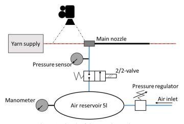
Figure 1: Sketch of the experimental setup.
