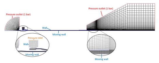
Figure 2: Mesh of the flow domain and its boundary conditions.
