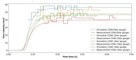
Figure 5: Experimental and simulated yarn velocity for a cotton yarn.
