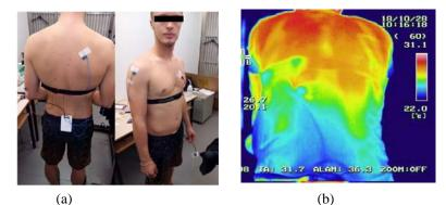
Figure 4. Receiver and sensors placed on the body (a) and thermal image of the back during the test
