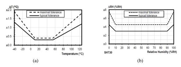
Figure 2. Tolerance of the temperature and humidity SHT31D sensor [SHT31D Datasheet]
