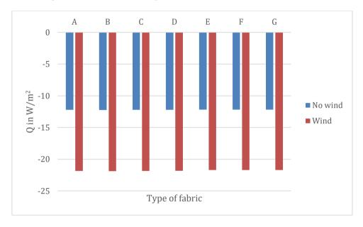
Figure 2. Heat transfer as a function of fabric type and wind.
