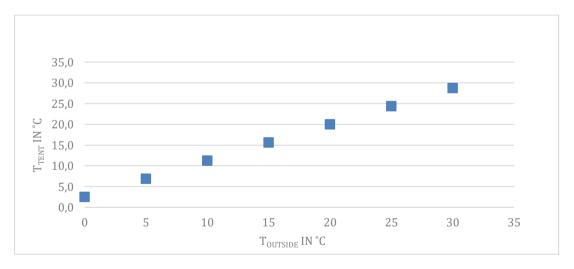
Figure 4. Temperature inner tent surface  $T_{tent}$  as a function of outside air temperature  $T_{outside}$
