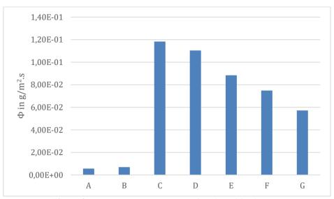
Figure 3. Water vapour transport as a function of fabric type.
