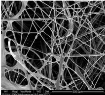
Figure 3. SEM image of PHA-based nanofibers
