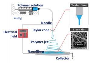
Figure 1. A basic electrospinning set-up
