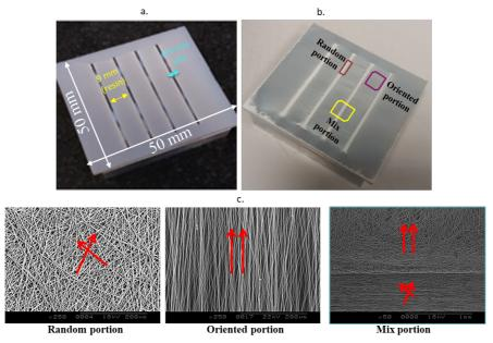
**Figure 2.** a.) characteristic of the hybrid collector with the respective dimensions, b.) fabricated patterned electrospun scaffold on the collector, c.) three different organization of nano-filaments on the collector
