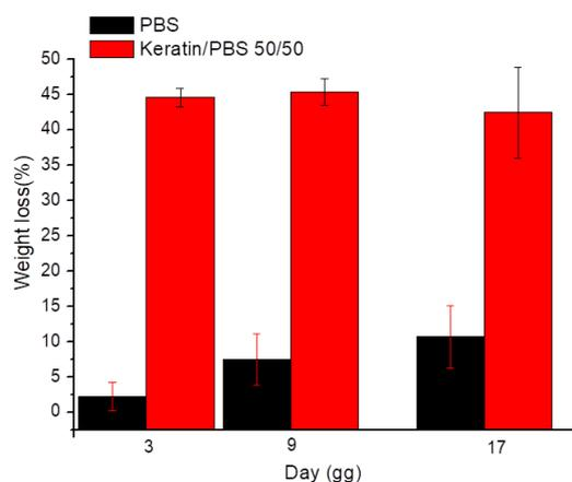
**Figure 3.** Weight loss of the samples evaluated under physiological conditions (pH 7.4 and 37°C) and in the presence of trypsin (2.5µg per mg of the sample).
