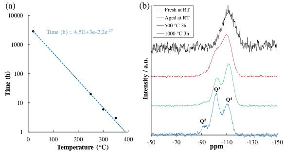
Figure 5. (a) Evolution of the heating time required for obtaining a superhydrophilic membrane as a function of the treatment temperature. The heating time increases exponentially upon lowering the heating temperature.
