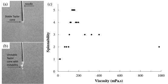
Figure 2. Electrospinnability of TEOS-based sol-gels by following the stability of the Taylor cone over time. Visualization of the Taylor cone: (a) Stable Taylor cone, (b) unstable, branched Taylor cone. (c) Electrospinnability as a function of the viscosity shows an optimal range between 120 and 200 mPa.s.
