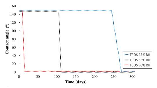
**Figure 4.** Water contact angle of silica nanofibers stored under controlled conditions of 20°C and 25, 65 and 90% RH. Just after the electrospinning the membrane is highly hydrophobic, with a contact angle around 150°. By storing the membrane under dry conditions, the hydrophobicity can be maintained for several months.
