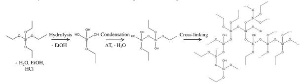
**Figure 1.** Principle of sol-gel synthesis for the direct electrospinning of silica nanofibers: the first step is an exothermal hydrolysis of the TEOS precursor, after which external heat allows for further condensation, resulting in a loosely cross-linked electrospinnable silica structure.
