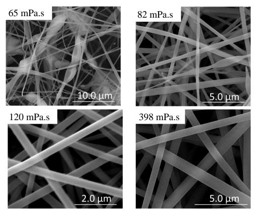
Figure 3. SEM images of silica nanofibers produced by direct electrospinning of a TEOS-based sol-gel system
