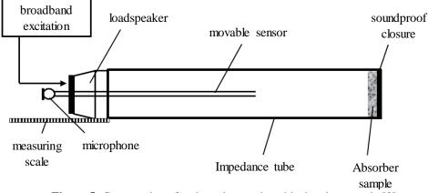
Figure 5: Construction of an impedance tube with absorber sample [3]
