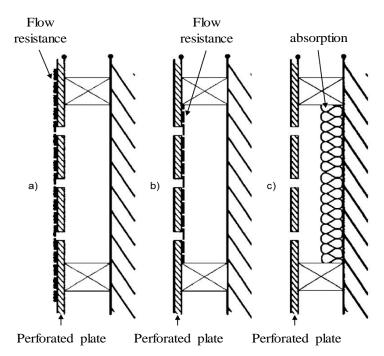
**Figure 4:** Helmholtz resonators of classical design with damping (c) in the cavity or flow resistance (a) in front or (b) behind the perforated plate [7]
