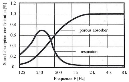
Figure 3: Principle frequency curve of sound absorption coefficient a of porous absorbers and resonators [2]
