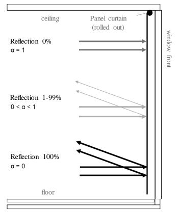
Figure 2: Principle of reflection and sound absorption coefficient [3]
