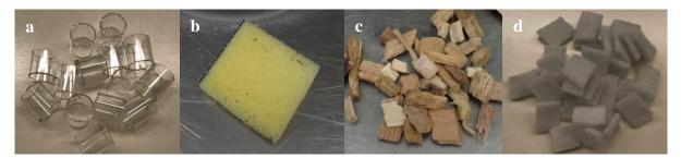
Figure 1 Images of packing materials: Raschig rings (a), PU foam (b), beech wood (c) and PES nonwoven (d)
