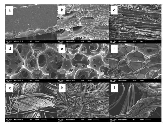
Figure 2 SEM images of surface morphology of Raschig ring corss-section (a), beech wood chip cross-section (b), eucalyptus wood chip (c), hard (d) and soft (e) PU foam, polyisocyanurate-based foam (f) and polyester woven (g), nonwoven (h) and 3D (i) textile.
