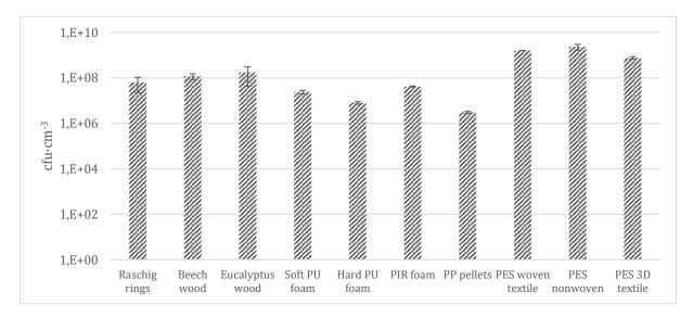
Figure 3 Biofilm formation of C. Necator (cfu·cm<sup>-3</sup>) in each packing material..
