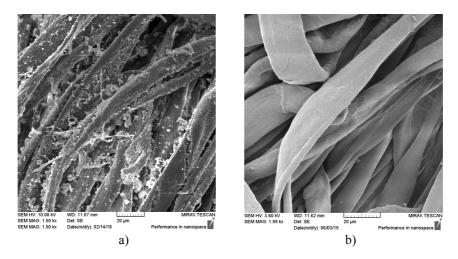
**Figure 2.** SEM micrographs of cotton fabric treated with Vibroactivated Zeolites –VZ\_5 (a) and Waterglass-WG10 (b)
