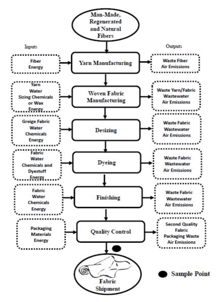
Figure 2. Flow diagram of investigated mill fabric production
