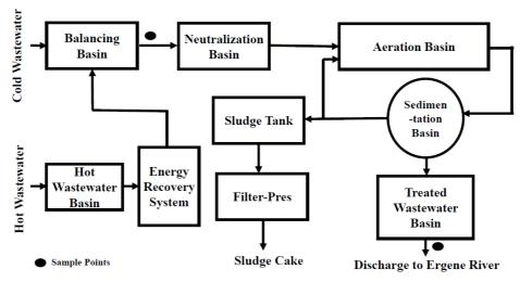
Figure 3. Flow diagram of investigated mill wastewater plant
