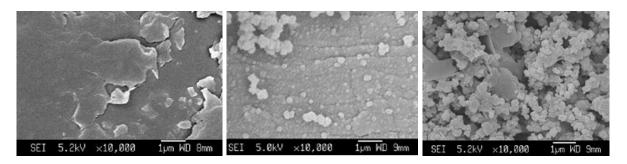
Figure 3. Initial membrane (top left), membrane coated with the application of iron chloride (top right) and with ammonium persulfate (bottom)
