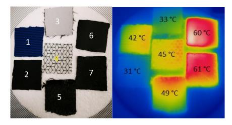
Figure 4. 1 – polyester/nylon 60/40 fabric with 20% graphene oxide; 2 – polyester lining fabric black colour; 3 – polyester shell fabric with white PU membrane; 4 – polyester fabric with 40% coverage print containing 18% graphene; 5 – pure carbon fiber fabric; 6 - polyester shell fabric with white PU membrane coated by polypyrrole; 7 – polyester fabric with PU membrane containing 18% of graphene oxide.
