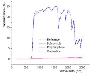
Figure 2. Transmittance of fabric with membrane coated with different polymers
