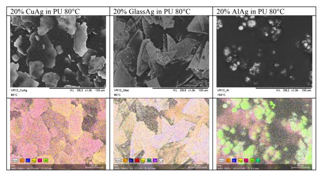
Table 1: SEM images and EDS of coatings with 20% particles in PU-dispersion dried at 80°C
