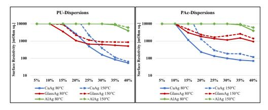
Figure 1: Influence of type of particle and concentration in PU- and PAc-Dispersions on surface resistivity
