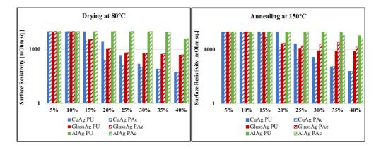
Figure 2: Influence of drying temperature for particles in PU- and PAc-dispersions on surface resistivity
