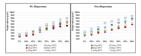
Figure 3: Correlation of weight add-on and concentration of particles in PU- and PAc-dispersions
