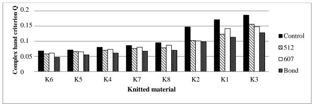
Figure 3. Complex hand criterion Q of the investigated knitted fabrics and their assemblies
