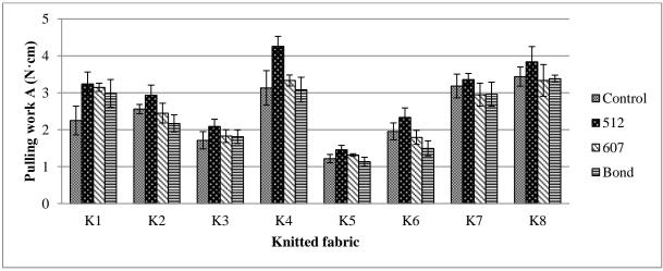
Figure 2. Pulling work A of the investigated knitted fabrics
