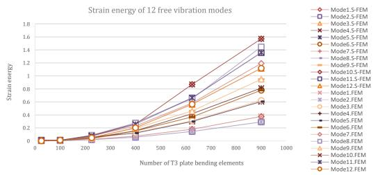
Figure 1. The strain energy of 12 free vibration modes between the implemented CS-FEM model and FEM for clamped edge boundary conditions with different mesh density.
