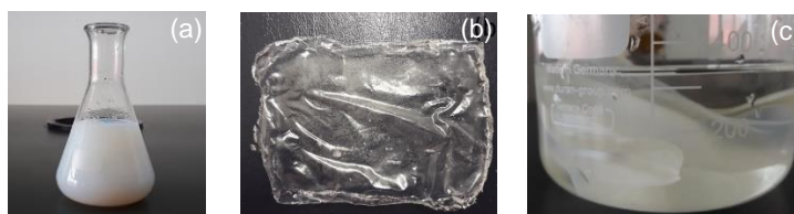
Figure 1. Acrylic emulsion (a), Chitosan/acrylic laminate film (b), Water uptake of chitosan/acrylic laminate film
