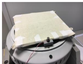
Figure 3. Measuring device for testing vibration isolation in the laboratory of BME
