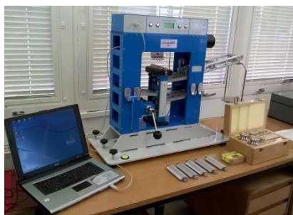
Figure 2. Cut resistance testing device in the laboratory of INNOVATEXT
