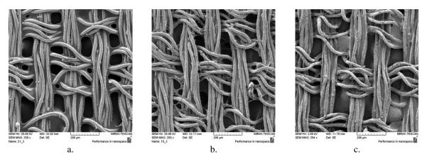
Figure 2. SEM images of polyamide fabrics metallized with copper: a. untreated; b. after 10 dry cleaning cycles; c. after 10 wet cleaning cycles
