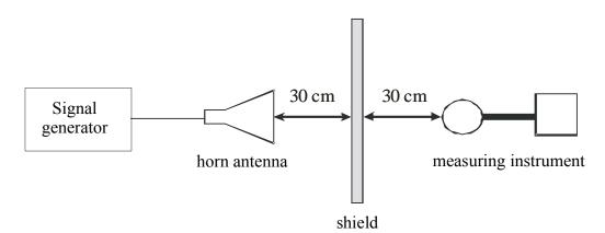
Figure 1. Measurement setup
