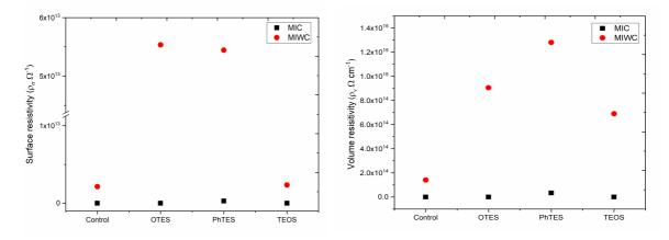
Figure 2. (a) Surface resistivity of MIC and MIWC samples, (b) Volume resistance of MIC and MIWC fabrics.
