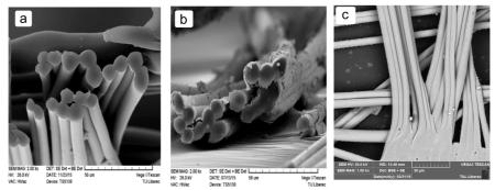
Figure 1. (a) Cross section views of MIWC, (b) MIC (before sol-gel coating), (c) MIC after PhTES coating.
