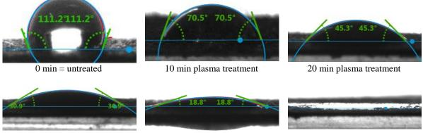
30 min plasma treatment40 min plasma treatment50 min plasma treatmentFigure 1. Examples of measurement of contact angle for evaluation of plasme treatment effect
