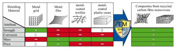
Figure 3. Substitution of common electromagnetic shielding materials by recycled carbon fibres
