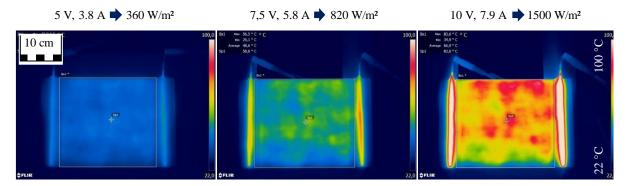
Figure 1. Sample plates of reinforced plastics from recycled carbon fibres as heating unit
