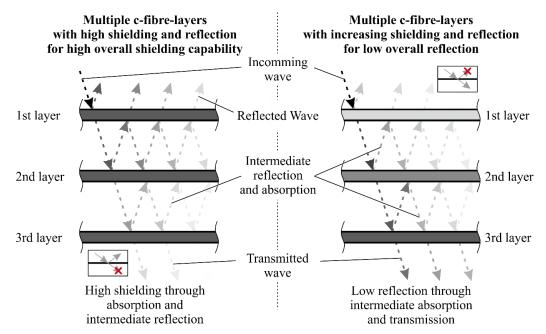
Figure 4. Optimisation of electromagnetic shielding, reflection and absorption by use of sandwich structures
