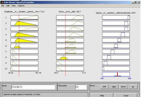
Figure3.Inference of the fuzzy decision system for determining the speed of operation of embroidery machine
