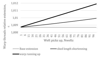
Figure 3, Variation of the warp threads extension during handloom weaving
