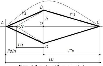
Figure 2, Parameters of the weaving shed
